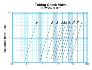
WATER FLOW RATE - GPM
