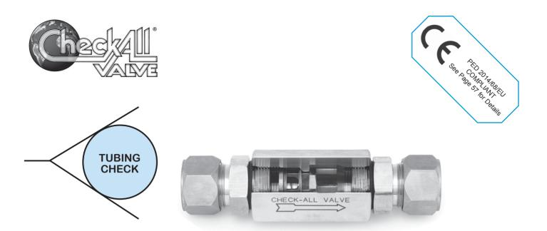
The **Tubing Check (TV)** valve is constructed with compression tube fittings (flareless) and is designed for a minimum pressure drop. The valves are furnished complete with ferrules and nuts. The TV valve can also be used as a low pressure relief valve or vacuum breaker by using the desired spring settings.
