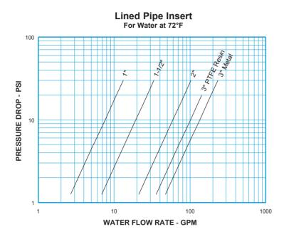
**Note:** All flow curves and Cv values presume the valves are fully open with 1/2 PSI cracking pressure springs. Consult the factory for more information.
